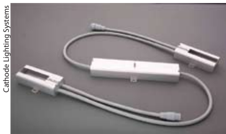
A contemporary, integrally ballasted "plug and play" cold cathode fixture (shown without lamp installed), which accepts a variety of lamp sizes and shapes
